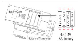
Open the battery cover of the transmitter and place the same type of battery with saturated capacity according to the '+-' electrode indication in the battery cell. (battery not included)
